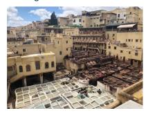
Chouara Tannery Using tanning methods unchanged since medieval times, the tannery operates without the use of machinery. It's an amalgam of stone vessels, some filled with white liquids made from various mixtures of cow urine, pigeon feces, quicklime, salt, and water in order to clean and soften tough animal skins, and others filled with natural dyes like poppy, indigo and henna used to color the hides before being laid to dry under the sun and sold and reworked into fine leather products.
